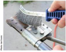
Cleaning: Keep the knife blade clean using a wire brush, always brush away from the gas jet with air and a solvent. It is advisable to carry two or three spare clean jets in a small, sealed container with other mulesing equipment.
